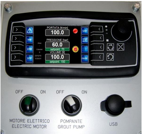
LCD Control panel (optional) with recording system and preset volume / pressure injection control
