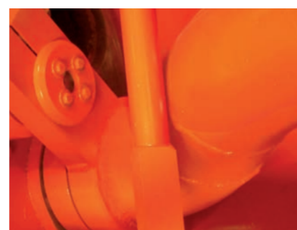
Tolva con válvula "S" con disco y placa de desgaste Hopper with "S" valve with disc and wear plate
