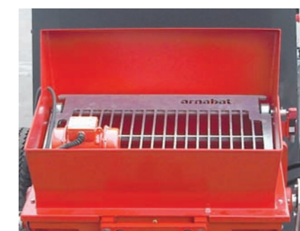
Rejilla para hormigón con electrovibrador Grill for concrete with electric vibrator
